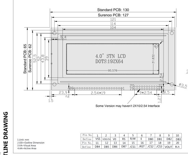
0.05 SHENZHEN SURENOO TECHNOLOGY CO.,LTD. 深圳市襄诺科技有限公司 REV0 1'ST DESIGN DATE: 2012013 WG TITLE: OUTLINE DRAWIN REV1 DWG NO.: 001 DESIGNED BY: JIM DATE REV2 SCALE: SLG19264B Series CHECKED BY: LGP NO.: 1 OF 1 APPROVED BY UNIT: MM CONFIRMED BY DATE: 2012/08/24
