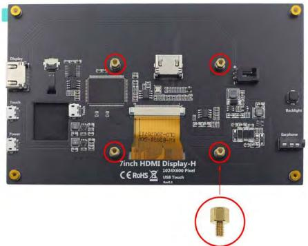
2) Place raspberry Pi and Install 4 Screws(M2.5)
